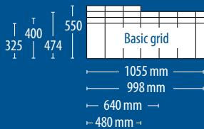
A joint basic raster depicts the drawer sizes and module variants. The drawers (blue) - depending on the raster involved - can be individually combined with the tool and distance modules (in colour). Appropriate configuration examples are on Page 005.
