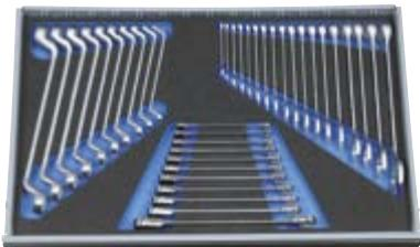
Double-ended ring spanner UD profile No. 2, AF 6x7 8x9 10x11 12x13 14x15 16x17 18x19 20x22 21x23 24x27 mm
